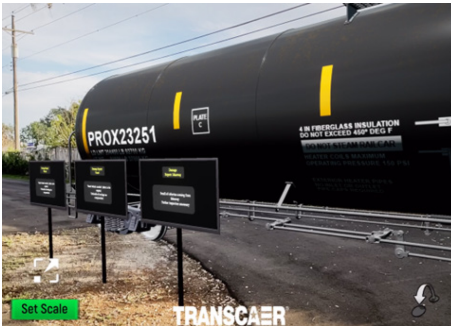
Figure 1: Example image for the TRANSCAER AR Training application with a computer generated, near full-scale railcar projected into the local real-world environment.
