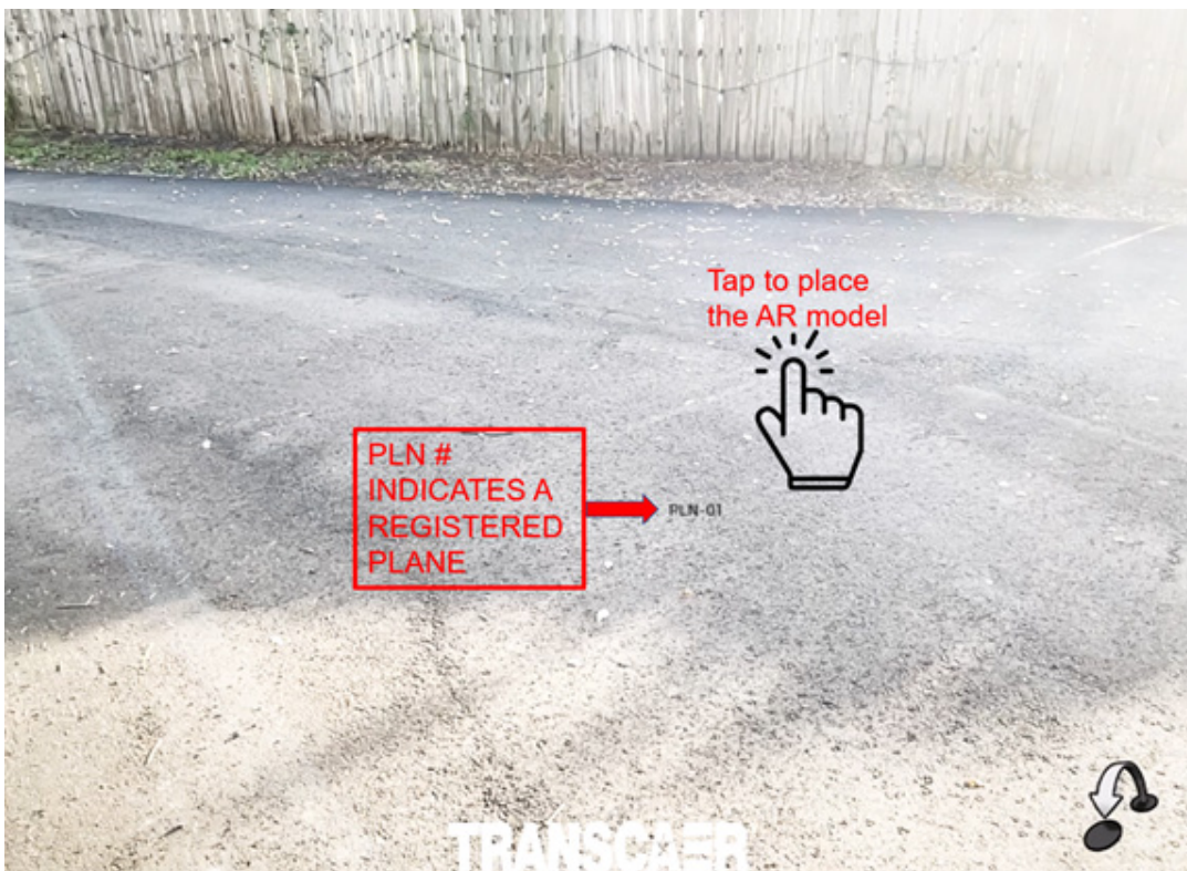
Figure 10: Camera view with PLN number to indicate that the application has recognized and registered the alley road as a surface plane where the AR model can be placed.
