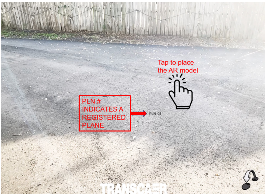
Figure 18: Camera view with PLN number to indicate that the application has recognized and registered the alley road as a surface plane where the AR model can be placed.
