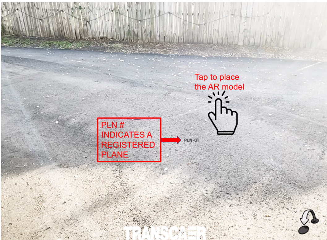
Figure 14: Camera view with PLN number to indicate that the application has recognized and registered the alley road as a surface plane where the AR model can be placed.
